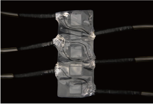
Figure 7: The water pouch used in the user test has three chambers so that it can change the size and the position of thermal stimulation.
