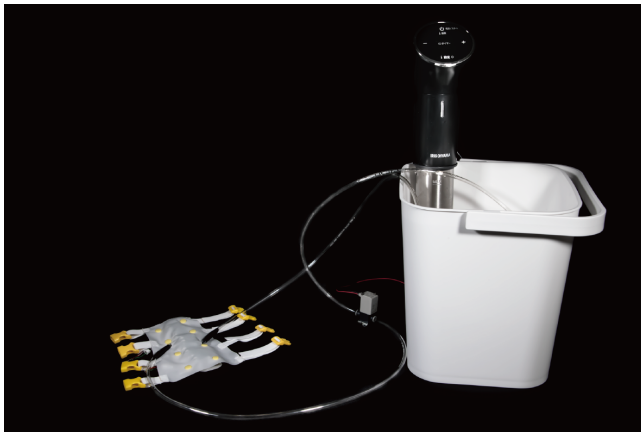
Figure 5: ThermoCaress (left) is connected to a water source (right) with tubes.
